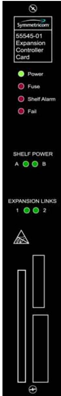
Figure 5-8. Front Panel of the Expansion Controller Card
