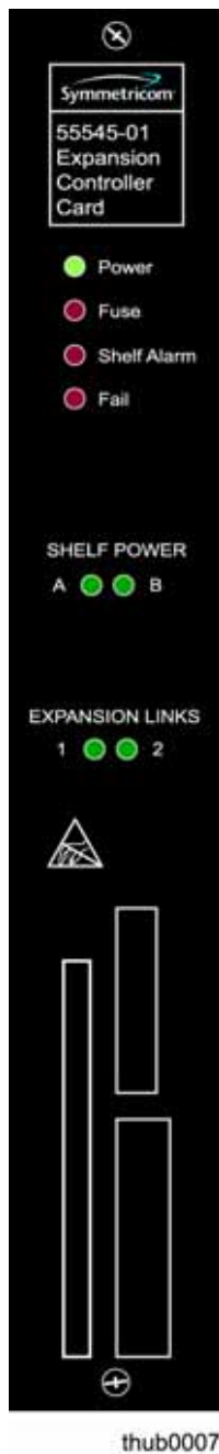
Figure 2-11. Front Panel of the Expansion Controller Card
